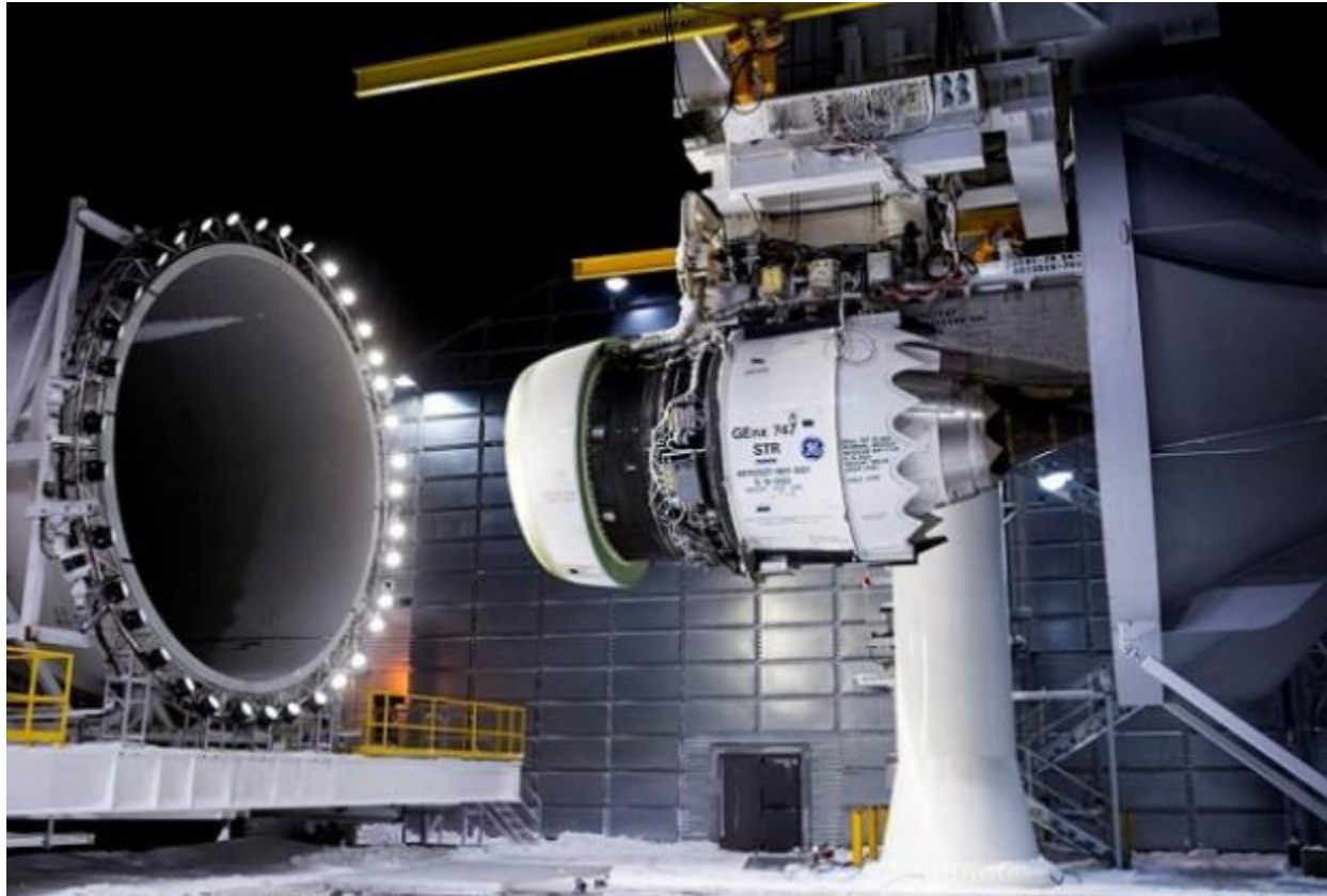
Image: At GE Aviation's testing facility in Winnipeg, GE engineers submit the GENx engine to cold weather tests that ensures the engine's performance in the harshest winter conditions.
